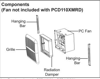
Note: Fan shown is not the PCD110XM or PCD110XMH
