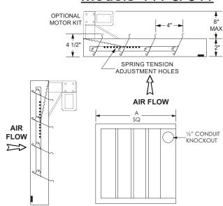
For low velocity (CFM) field adjustment a spring tension may be required to ensure that damper blades open completely.
