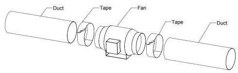
The ducting from this fan to the outside of the building has a strong effect on the air flow, noise, and energy use of the fan. Use the shortest, straightest duct routing possible for the best performance, and avoid installing the fan with smaller ducts than recommended. Insulation around the ducts can reduce energy loss and inhibit mold growth. Fans installed with exisiting ducts may not achieve their rated flow.
