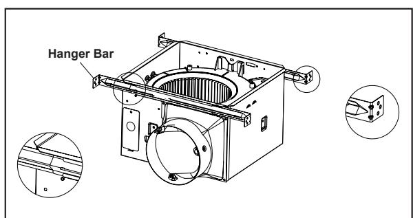
2. Extend the hanger bars to the width of the framing. Position the ventilator with the bottom edge of the hanger bar tabs are flush with the bottom edge of the framing, holding the ventilator in place. Secure hanger bars to framing using one screw on each end of hanger bar. Select a proper hole and secure the hanger bars together using one screw.
