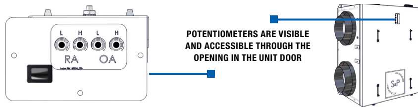
FIGURE 4.5.1 FAN SPEED CONTROL POTENTIOMETERS
